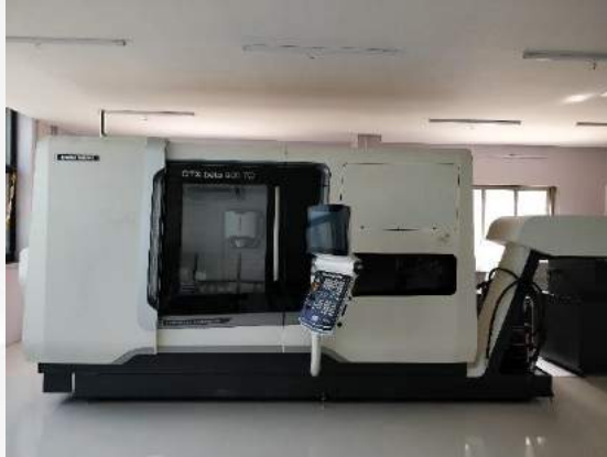
Multitasking Machines, with \varnothing 500mm Turning Dia. & 800 mm Long Machining capability
