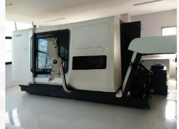
Multitasking Machines, with \varnothing 500mm Turning Dia. & 800 mm Long Machining capability
