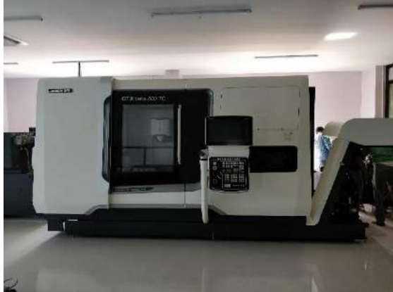
Multitasking Machines, with \varnothing 500mm Turning Dia. & 800 mm Long Machining capability
